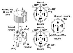
Figure 18 - Cord and Plug Configurations
